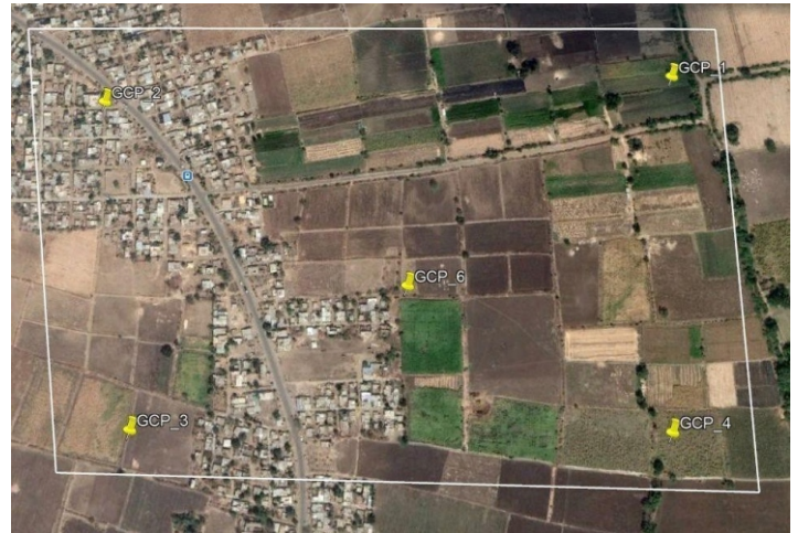
Figure: Drone AOI with GCP placement
